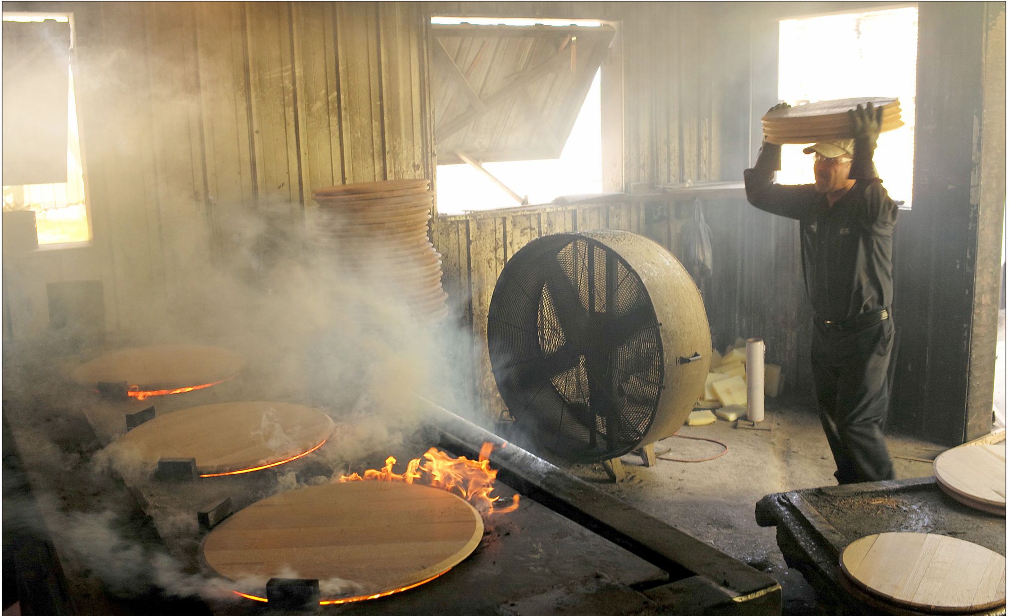
Luis Viramonte has been charring barrel heads in the furnace room of the McGinnis Wood Products Company for six years. The process of charring the inside of the barrels by flame adds flavor to bourbon. The job is one of the toughest in the factory that produces white oak bourbon barrels that are shipped throughout the world.
